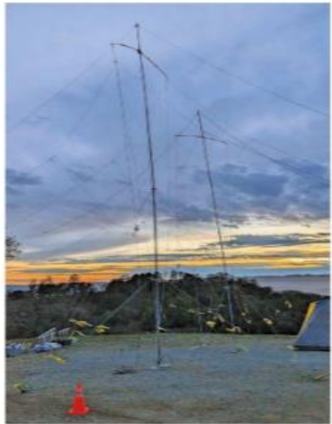
Figure 1 — Use yellow or orange safety tape to flag all of the guy lines, and place traffic cones to keep vehicles in a safe place. [Steve Sergeant, KC6ZKT, photo]
