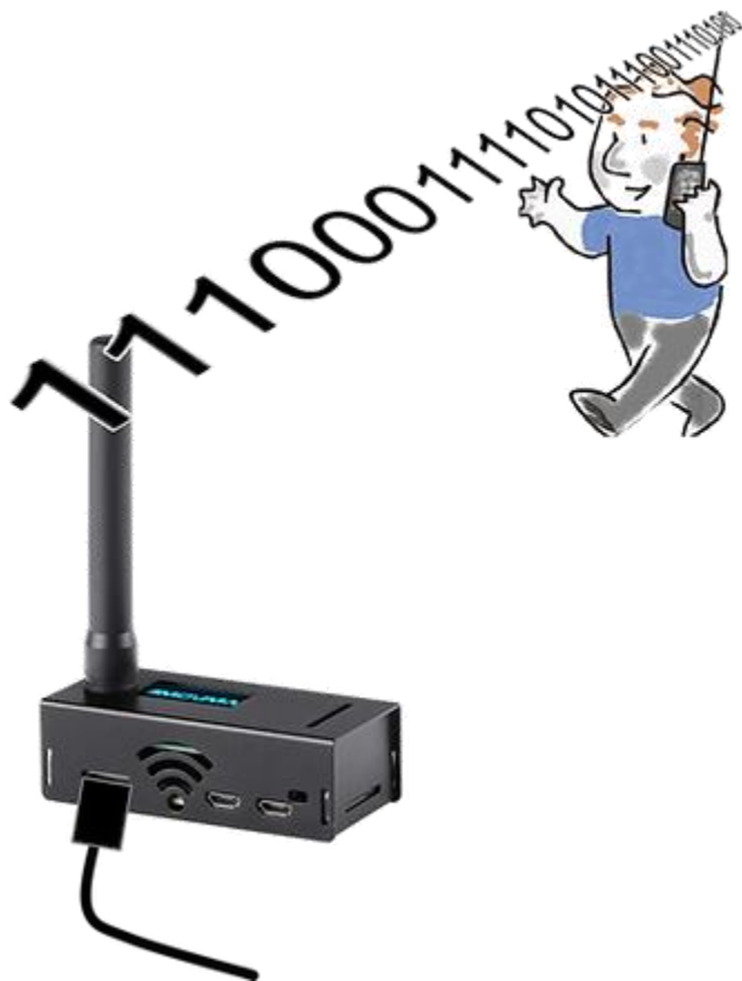
Figure 4. Typical hotspot use is a handheld transceiver communicating locally to a low-power hotspot connected to the internet.
